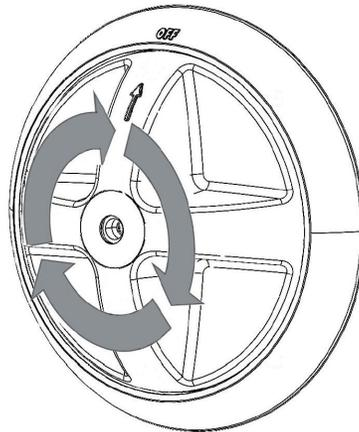
11. Insert screw cover with o-ring installed, into recess of handle.
