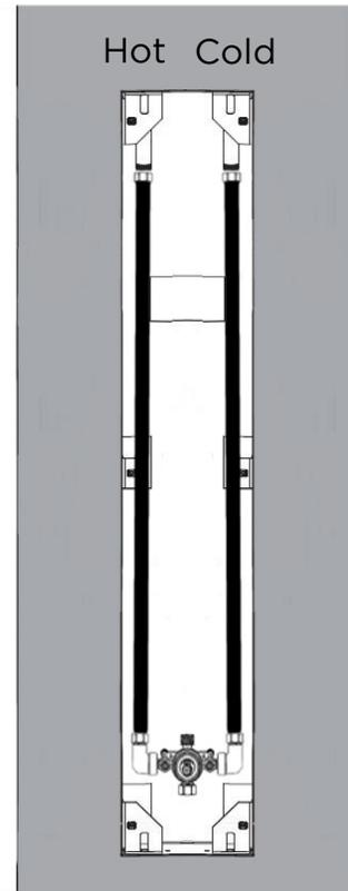
12A. **Install the hose for the connection from the valve to the shower head.**
