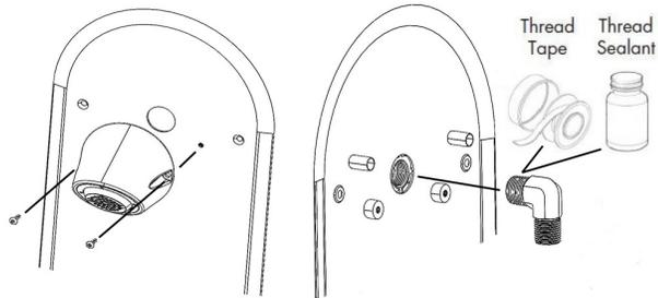
**Important:** Use thread sealing tape or liquid pipe thread sealant on the shower head to elbow connection to prevent leaks.
