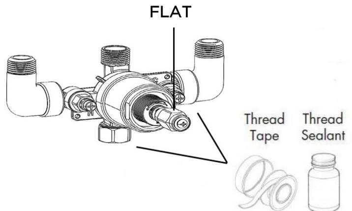
**Important:** Use thread sealing tape or liquid pipe thread sealant on the elbow to valve connection, and the cap to valve connection, to prevent leaks.
