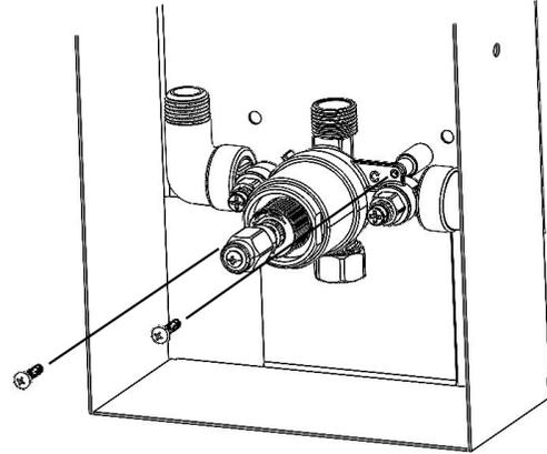
7. Place the wall plate over the hole on the front panel. Orient the wall plate so the "OFF" marking is at the top position as shown below. Secure wall plate to the front panel with the 1" Phillips screws provided.
