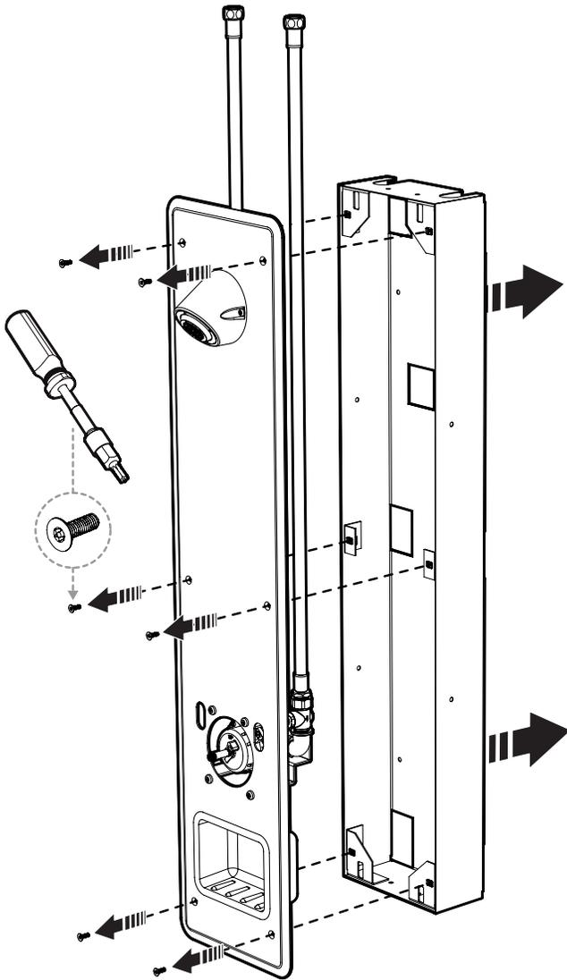
2. Measure and cut hole in wall where the cabinet is to be installed. Ensure proper mounting structure is present within the wall to support the unit in use.
