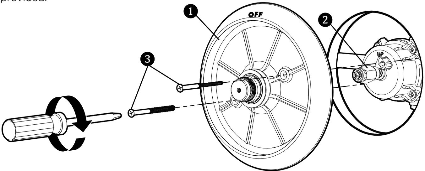
10. Verify that the Friction Ring is properly seated into the Friction Ring Groove of the Wall Plate.
